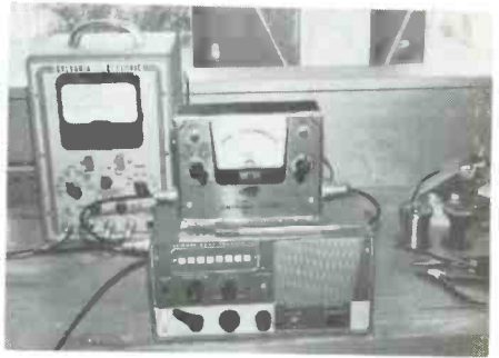
In-Line Wattmeter Can Be Used To Check SWR, Outgoing Watts, and Reflected Watts.
